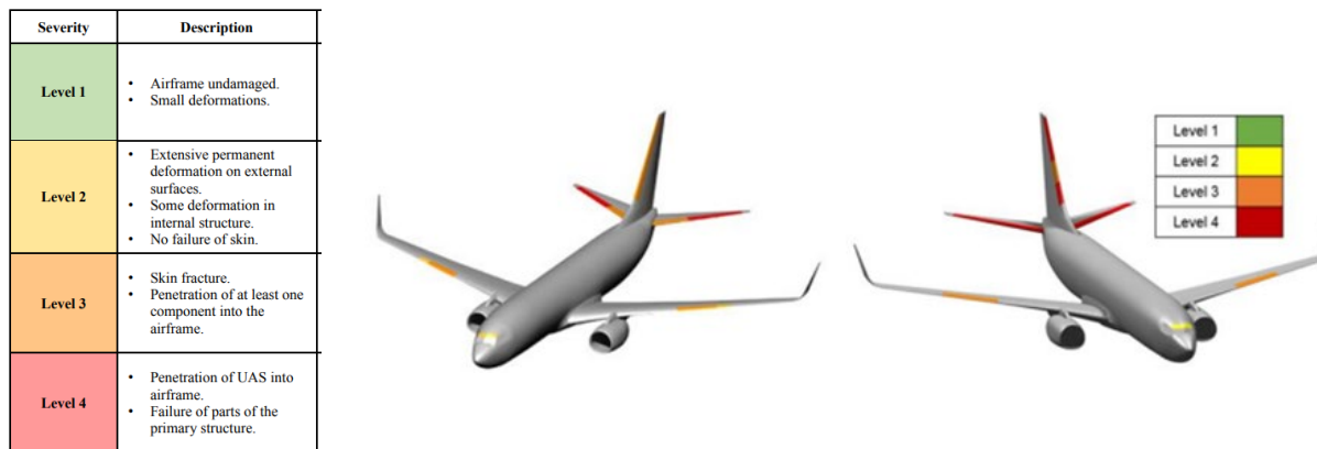
Fig. 3: The damage level categories and the aircraft consequence of a 1.2 kg quadcopter collision (left) or 1.8 kg collision with a fix wing (right) drone collision severity levels on commercial transport jet type aircraft
