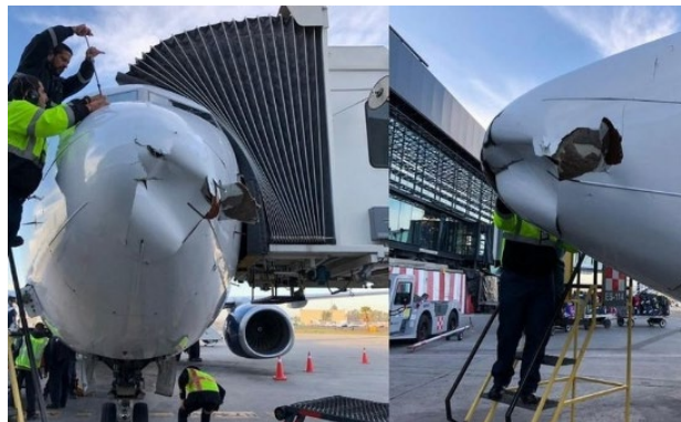
Fig. 2 : The damaged nose of Aeromexico's 737 jet 5
